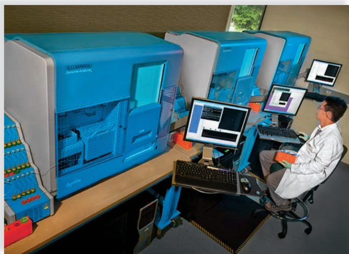
Figure 21.14 Automated DNA sequencer and an electropherogram.
